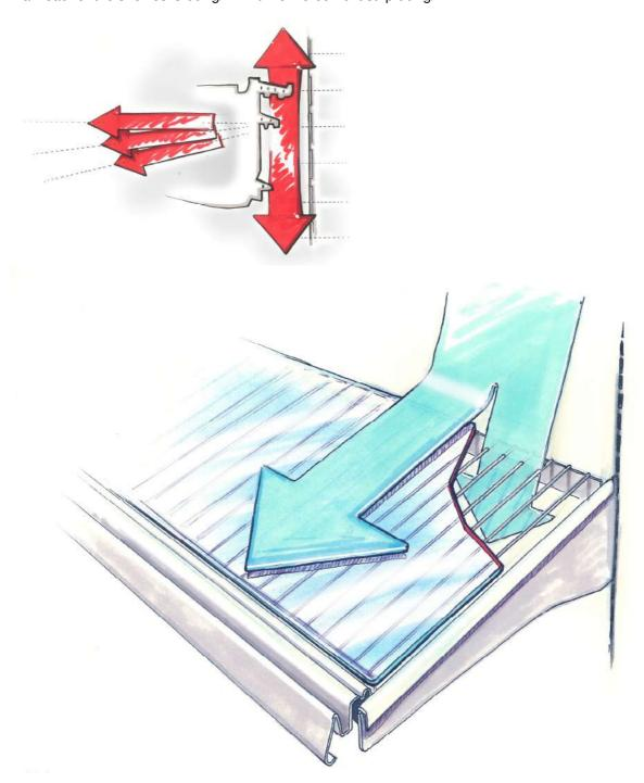
If shelf grid is used a transparent persplex layer is required to distribute the cold air in the correct way.
